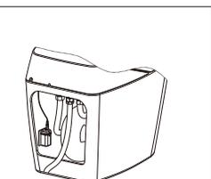
④ Remove the label of sticker and fix the battery box to the ceramic toilet.
