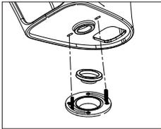
5. Put the flange sealing ring on the flange, and then align the mounting bolts through the mounting holes at the bottom of the toilet.
