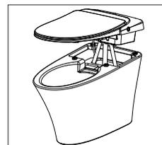
4. Lift the cover up a little from the back of the toilet, so that you can loosen the braided tube and wires behind the electronics cover.
