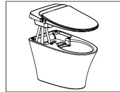
8. Adjust the position of the upper cover, align it with the 4 installation holes of the ceramic body, press down firmly, and the installation is complete.
