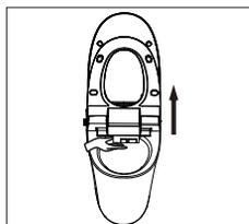
3. Separate the electronic seat cover with the ceramic by holding the upper cover with both hands and lift it up.
