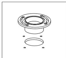
1. According to the position of the four screw holes of the flange, make four holes around the floor drain outlet, and drive in expansion screws to fix the flange.
