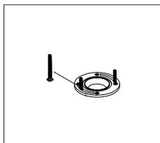
2. Insert the toilet mounting bolts into the grooves of the flange, then align the flange with the sewage outlet and tighten the screws to fix it.
