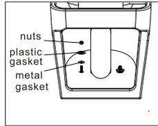
6. Put metal gaskets, plastic gaskets and nuts on the bolts in sequence, and then tighten the screws to fix them after the installation is stable. (Please process this installation from the top of the toilet bowl )
